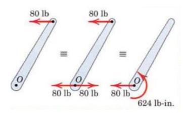
We apply two equal and opposite 80· lb forces at O and identify the counterclockwise couple
