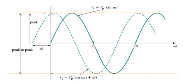
Figure (1): Illustrating for sinusoid signal attributes
