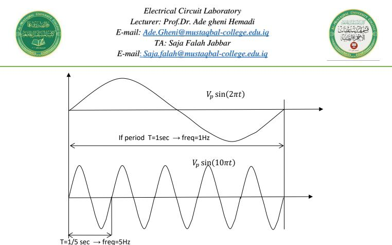
From above figure it's obvious that signal period is reciprocal of its frequency. Finally the phase shift between any two equal frequency signals ( $\emptyset$ ).
