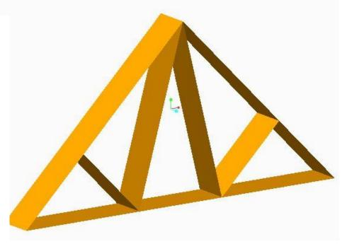
Trusses consist of triangular units constructed with straight members.
