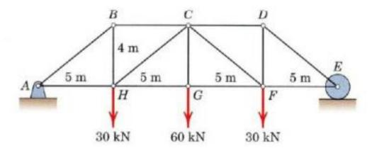
As a whole:  $\Sigma F_{\chi} = 0 \Rightarrow A_{\chi} = 0$ (Dim. in m) 19 x Ay = E = 60 KN by IFy = 0 and symmetry.  $(\theta = \tan^{-1}(\frac{4}{5}) = 38.7^{\circ})$ Joint A: SEx=0:-BC+96.0 sin 51.3°=0, BC=75 kN C EFy=0:-BH + 76.0 cos 51.3°=0, BH= 60 KNT 96.0 KN BH [ EFy=0:-CH sin 0+30=0, CH=48.0 KN C (ZFx=0:-48.0 cos+ GH-75=0 GH = 112.5 kN T 75 kN XFy =0 > CG = 60 KN T Joint G: By symmetry: FG= 112.5 kNT, CF 48.0 kN C CG 1 CD = 75 KN C. DF = 60 KN T 112.5 EF = 75 KNT, DE = 96.0 KN C
