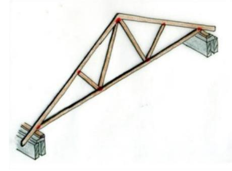
• A truss is made up of a web of triangles joined together to enable the even distribution of weight and the handling of changing tension and compression without bending or shearing. The triangle is geometrically stable when compared to a four (or more) -sided shape which requires that the corner joints are fixed to prevent shearing.
