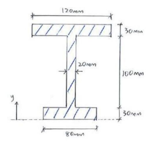
Find the centroid  $\bar{\mathbf{y}}$  of the unsymmetrical I-section with respect to its base.
