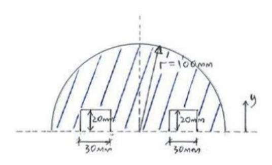
Calculate the centroid  $\bar{\mathbf{y}}$  of the geometry with respect to its base.
