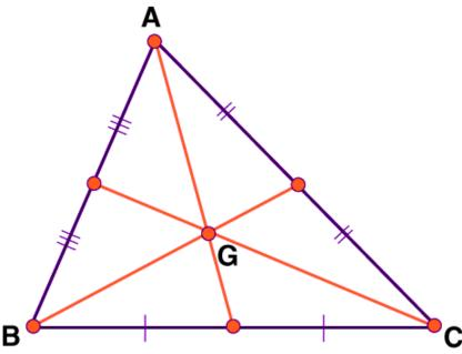
• The center of mass equal to centroid if the body is homogeneous.
