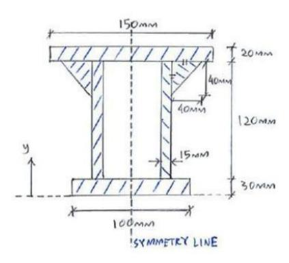
Calculate the centroid  $\bar{\mathbf{y}}$  of the geometry with respect to its base.
