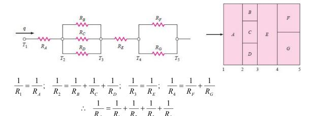
$R_{th} = R_1 = R_2 = R_3 = R_4$  ( $R_{th}$  is the thermal resistances)
