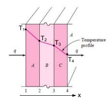
The heat flow must be the same through all sections, therefore,
