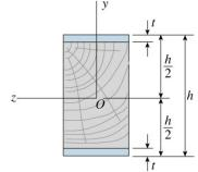
$$M = - \int_{A} \sigma_{x} y \, dA = - \int_{1} \sigma_{x1} y \, dA + - \int_{2} \sigma_{x2} y \, dA$$
