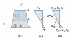
this equation can be used to located the N. A. of the cross section for beam of two materials, the integrals represent the 1<sup>st</sup> moment of two parts w. r. t. the N. A.
