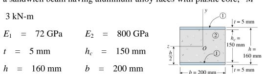
determine  $\sigma_{max}$  and  $\sigma_{min}$  in the faces and core
