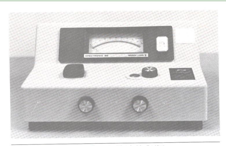
Figure 7–5. An example of a spectrophotometer (Photo by John Estridge)
