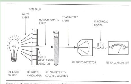
Figure 7-6. Diagram of internal parts of a spectrophotometer
