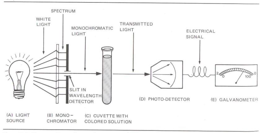
Figure 7–6. Diagram of internal parts of a spectrophotometer
