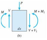
i.e. an abrupt change in the shear force occurs at any point where a concentrated load acts
