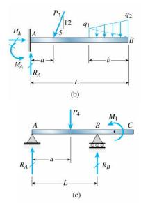
b. cantilever beam (fixed end beam)
