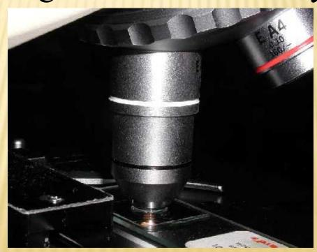
Clean up!: When you have finished for the day, wipe the 100x oil immersion objective carefully with lens paper to remove all oil. Wipe oil from the slide thoroughly with a Kimwipe. Cleanse stage should any oil have spilled on it. Recap the immersion oil container securely, replace in drawer.
