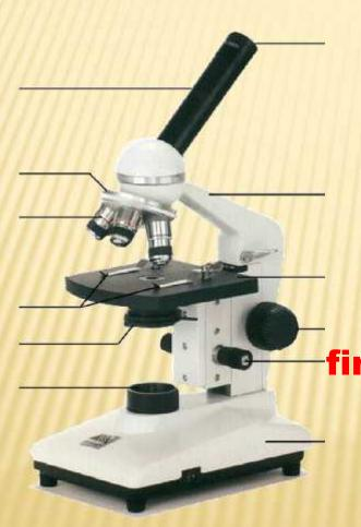
small, round knob on the side of the microscope used to fine-tune the focus of your specimen
