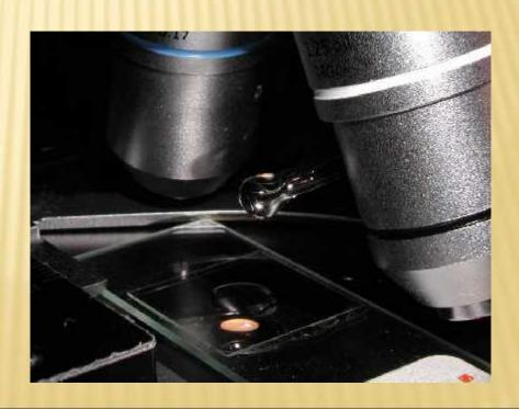
Rotate so that the 100x oil immersion objective touches the oil and clicks into
