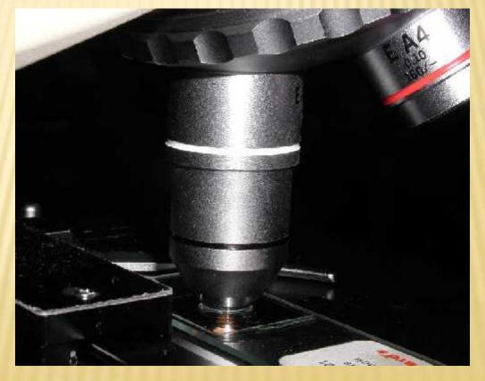
Focus **only** with fine focus. Hopefully, the specimen will come into focus easily. Do not change focus dramatically.
