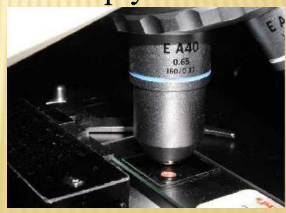
Partially rotate so that 40x and 100x objectives straddle the specimen.
