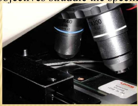
Place a small drop of oil on the slide in the center of the lighted area. (Take care not to dribble on the stage.)
