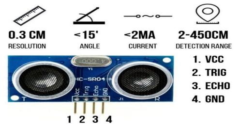
Ultrasonic Sensor HC-SR04 Configuration and Specification
