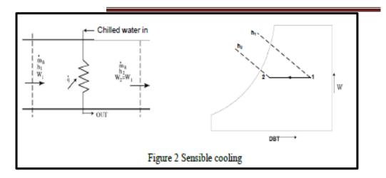
Calculate the cooling load when 1.5 m<sup>3</sup>/s of moist-air, initially at a state of 21 °C DBT, 15 °C WBT and 101.325kPa barometric pressure, 1 is cooled sensibly by 5 °C using cooler coil, what is the flow rate of chilled water necessary to effect this cooling if the flow return temperature of 10°C and 15 °C satisfactory.
