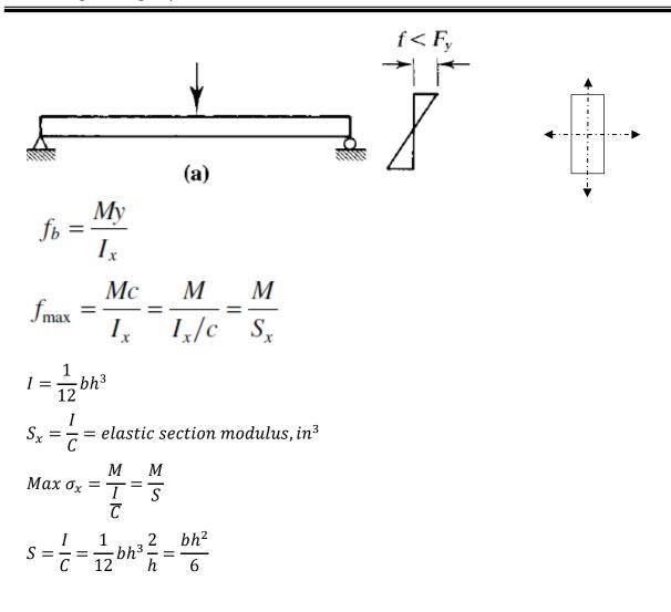
When  $Max \ \sigma_x = F_y$   $M = M_y = moment \ at the elastic liumit$   $F_y = \frac{M_y}{S}$  $M_y = F_y S$
