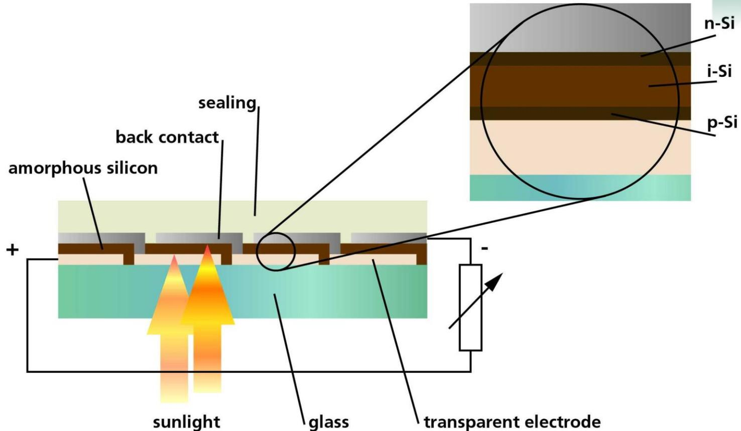
monolithic interconnection in an a-Si module
