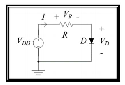
We will assume that the diode is forward biased. Using KVL
