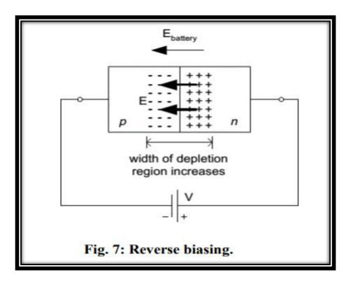
For the reversed biased state of the PN junction, the electric field produced by the battery E battery adds to this electric field of the space charge E in the depletion region. This increases the width of the depletion region. Consequently, the "majority carriers" cannot flow through the region: holes in the p material are opposed by E in the depletion region, as are electrons in the n material. Hence, little current flows (only the drift current  $I_S$ ) unless the junction breaks
