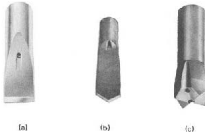
Figure 1.4: Chopping and jetting bits: (a) straight; (b) chisel; (c) cross. (Wash boring).
