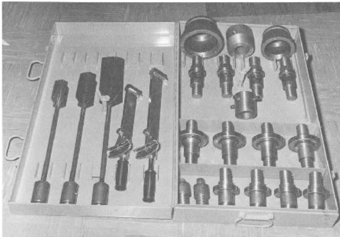
Figure 1.17: Vane shear equipment: vanes, torque wrenches, bushings for drill rods, and casing cap.
