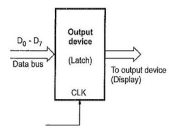
When microprocessor wants to send data to the output device, it puts the data on the data bus and activates the clock signal of the latch, latching the data from the data bus at the output of latch. It is then available at the output of latch for the output device.
