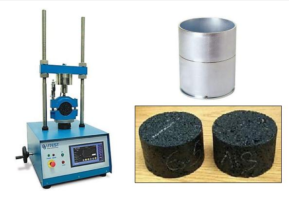
Stability: maximum load resistance of standard specimen (4" dia. & 2.5" height) when tested in the direction of diameter, at 60°C at the rate of 2"/min.
