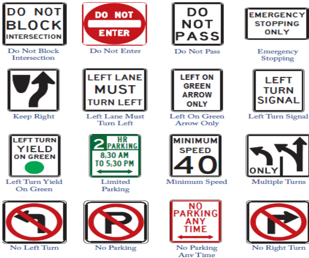
Figure 7 Traffic regulation signs
