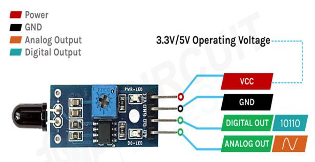
VCC Provides power for the module, Connect to the 5V pin of the Arduino.
