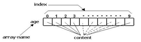
The item in an array are called elements (in contrast to the items in a structure which are called members). The elements in an array are of the
