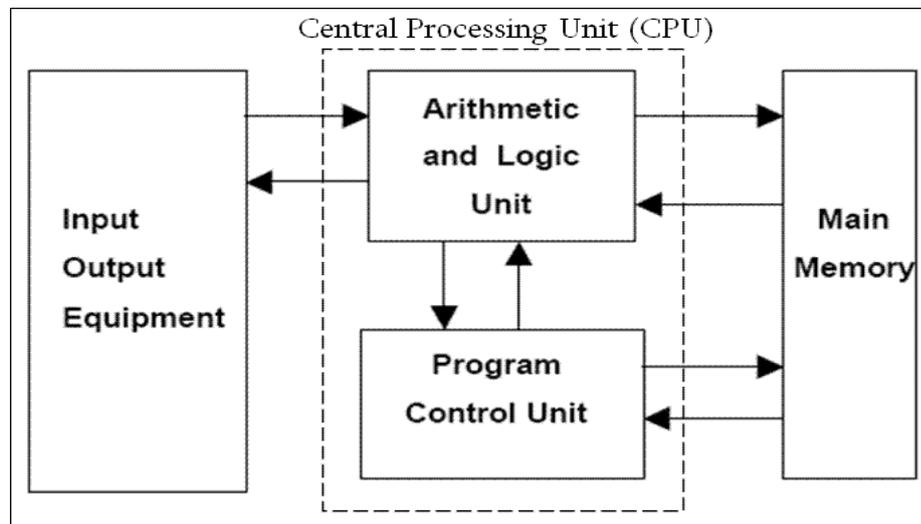
Figure : General structure of Von Neumann Architecture
