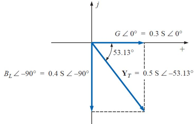
$$\mathbf{I} = \frac{\mathbf{E}}{\mathbf{Z}_T} = \mathbf{E}\mathbf{Y}_T = (20 \text{ V } \angle 53.13^\circ)(0.5 \text{ S } \angle -53.13^\circ) = \mathbf{10 \text{ A } } \angle 0^\circ$$
