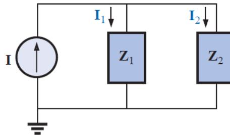
$$\mathbf{Z}_1 = R + jX_L = 3 \Omega + j4 \Omega = 5 \Omega \angle 53.13^\circ$$
