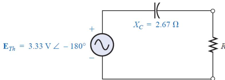
**EXAMPLE:** Determine the Norton equivalent circuit for the network external to the 6-Ω resistor.
