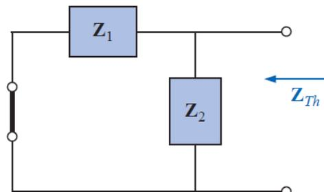
$$\begin{aligned} \mathbf{Z}_{Th} &= \frac{\mathbf{Z}_1 \mathbf{Z}_2}{\mathbf{Z}_1 + \mathbf{Z}_2} = \frac{(j 8 \Omega)(-j 2 \Omega)}{j 8 \Omega - j 2 \Omega} = \frac{-j^2 16 \Omega}{j 6} = \frac{16 \Omega}{6 \angle 90^\circ} \\ &= 2.67 \Omega \angle -90^\circ \end{aligned}$$
