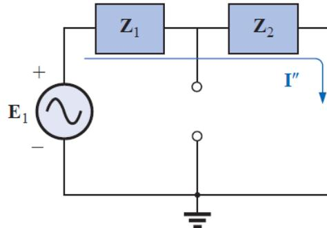
$$\begin{aligned} \mathbf{I}'' &= \frac{\mathbf{E}_1}{\mathbf{Z}_T} = \frac{\mathbf{E}_1}{\mathbf{Z}_1 + \mathbf{Z}_2} = \frac{20 \text{ V} \angle 30^\circ}{6.32 \Omega \angle -18.43^\circ} \\ &= 3.16 \text{ A} \angle 48.43^\circ \end{aligned}$$
