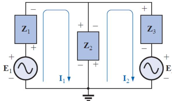
$$\begin{aligned} \mathbf{Z}_1 &= +jX_L = +j2 \Omega & \mathbf{E}_1 &= 2 \text{ V} \angle 0^\circ \\ \mathbf{Z}_2 &= R = 4 \Omega & \mathbf{E}_2 &= 6 \text{ V} \angle 0^\circ \\ \mathbf{Z}_3 &= -jX_C = -j1 \Omega \end{aligned}$$
