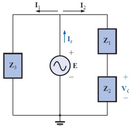
$$\begin{aligned} V_C &= \frac{Z_2 E}{Z_1 + Z_2} = \frac{(12 \Omega \angle -90^\circ)(20 \text{ V } \angle 20^\circ)}{5 \Omega - j 12 \Omega} = \frac{240 \text{ V } \angle -70^\circ}{13 \angle -67.38^\circ} \\ &= 18.46 \text{ V } \angle -2.62^\circ \end{aligned}$$
