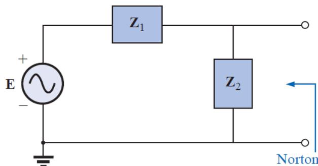
$$Z_1 = R_1 + j X_L = 3 \Omega + j 4 \Omega = 5 \Omega \angle 53.13^\circ$$
