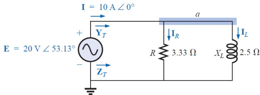
$$\begin{aligned} Y_T &= Y_R + Y_L \\ &= G \angle 0^\circ + B_L \angle -90^\circ = \frac{1}{3.33 \Omega} \angle 0^\circ + \frac{1}{2.5 \Omega} \angle -90^\circ \\ &= 0.3 \text{ S } \angle 0^\circ + 0.4 \text{ S } \angle -90^\circ = 0.3 \text{ S} - j 0.4 \text{ S} \\ &= \mathbf{0.5 \text{ S } \angle -53.13^\circ} \end{aligned}$$
