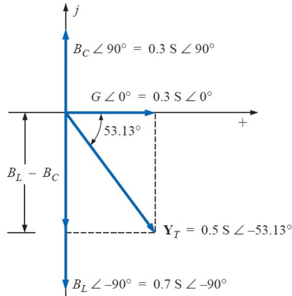
$$\begin{aligned} \mathbf{I}_R &= (E \angle \theta)(G \angle 0^\circ) \\ &= (100 \text{ V} \angle 53.13^\circ)(0.3 \text{ S} \angle 0^\circ) = \mathbf{30 \text{ A} \angle 53.13^\circ} \end{aligned}$$
