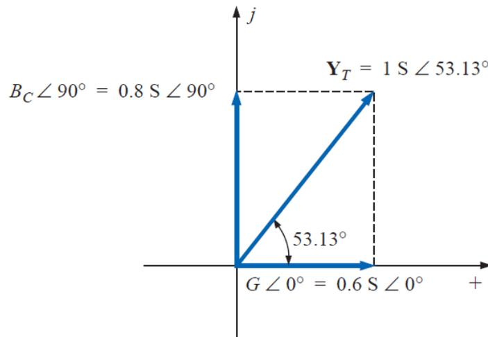
$$\mathbf{E} = \mathbf{I} \mathbf{Z}_T = \frac{\mathbf{I}}{\mathbf{Y}_T} = \frac{10 \text{ A} \angle 0^\circ}{1 \text{ S} \angle 53.13^\circ} = \mathbf{10 \text{ V} } \angle \mathbf{-53.13^\circ}$$
