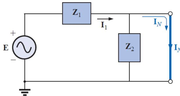
$$I_N = I_1 = \frac{E}{Z_1} = \frac{20 \text{ V} \angle 0^\circ}{5 \Omega \angle 53.13^\circ} = \mathbf{4 \text{ A} \angle -53.13^\circ}$$
