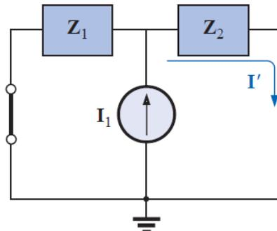
$$\begin{aligned} \mathbf{I}' &= \frac{\mathbf{Z}_1 \mathbf{I}_1}{\mathbf{Z}_1 + \mathbf{Z}_2} = \frac{(j 6 \Omega)(2 \text{ A})}{j 6 \Omega + 6 \Omega - j 8 \Omega} = \frac{j 12 \text{ A}}{6 - j 2} \\ &= \frac{12 \text{ A} \angle 90^\circ}{6.32 \angle -18.43^\circ} \end{aligned}$$
