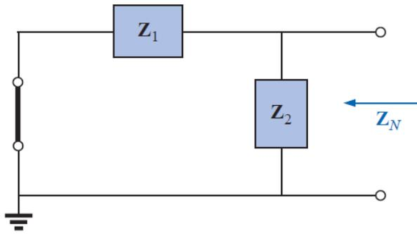
$$Z_N = \frac{Z_1 Z_2}{Z_1 + Z_2} = \frac{(5 \Omega \angle 53.13^\circ)(5 \Omega \angle -90^\circ)}{3 \Omega + j4 \Omega - j5 \Omega} = \frac{25 \Omega \angle -36.87^\circ}{3 - j1}$$
