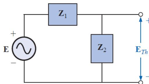
$$E_{Th} = \frac{Z_2 E}{Z_1 + Z_2} \quad (\text{voltage divider rule})$$
