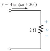
$$i = 4 \sin(\omega t + 30^{\circ}) \Rightarrow \text{phasor form } \mathbf{I} = 2.828 \text{ A} \angle 30^{\circ}$$
