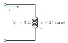
$$V = 24 \sin \omega t \Rightarrow \text{phasor form } \mathbf{V} = 16.968 \text{ V} \angle 0^{\circ}$$
