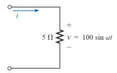
$$v = 100 \sin \omega t \Rightarrow \text{phasor form } \mathbf{V} = 70.71 \text{ V} \angle 0^{\circ}$$
