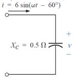
$$i = 6 \sin(\omega t - 60^{\circ}) \Rightarrow \text{phasor notation } \mathbf{I} = 4.242 \,\text{A} \, \angle -60^{\circ}$$
