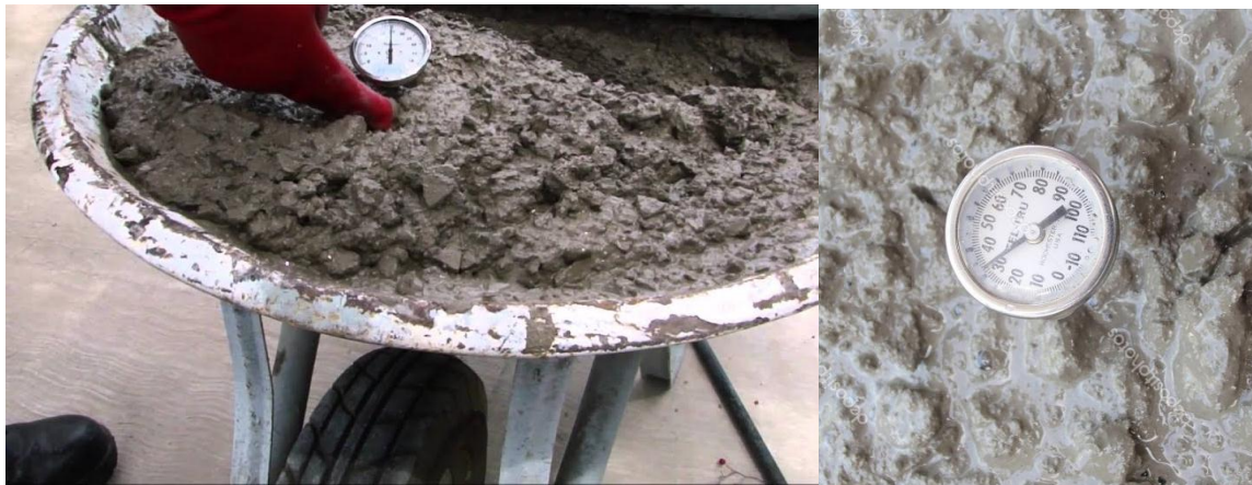
Fig.4: Temperature test of freshly concrete.
