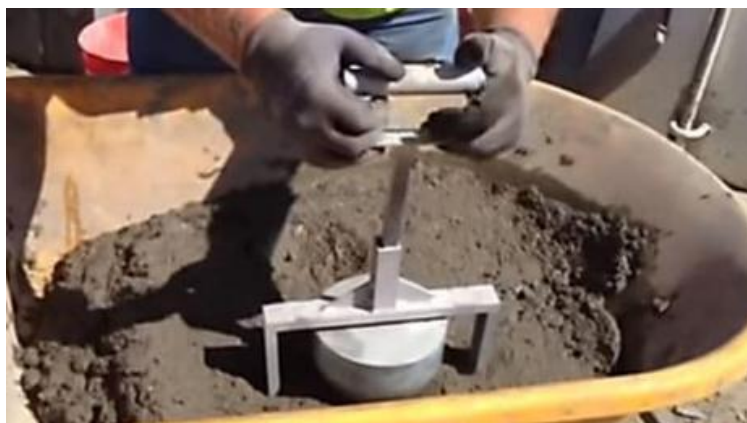
Fig.9: Performing kelly Ball Test.
