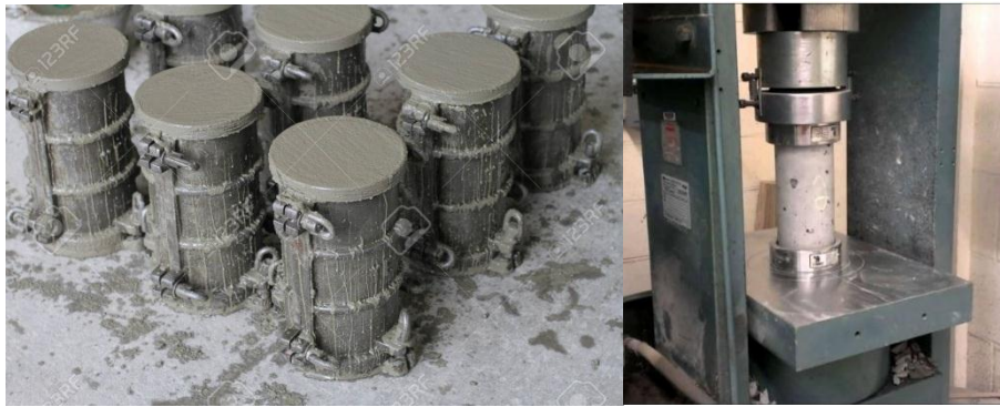
Fig.13: Casting Cylinder and Testing of Compressive strength of concrete.
