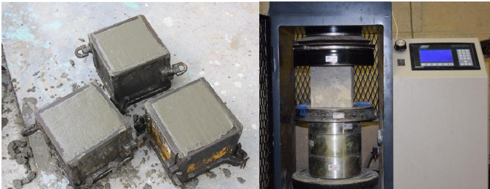
Fig.12: Casting cubes and Testing of Compressive strength of concrete.
