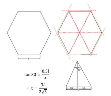
**EXAMPLE 19:** For the same hexagon shaped slab and subjected to the same loading, determine the ultimate resisting moment per linear meter if the supports are fixed at all sides.
