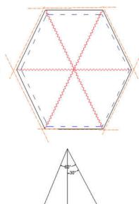
**EXAMPLE 20:** for the simply supported octagon shaped 2-way slab, using the yield line theory determine the resisting moment per linear meter (m) withstanding a uniformly distributed load of w.
