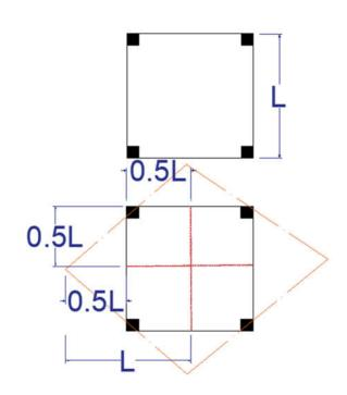
**EXAMPLE 24:** The two-way reinforced concrete slab is supported as shown in the figure below. Using the proposed moment proportions, determine the ultimate resisting moment per linear meter (m) using the yield line theory when the slab is subjected to a load of 12kN/m<sup>\*</sup>.
