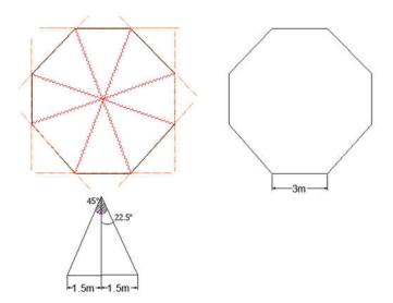
**Example 21:** The triangular simply supported two-way slab shown in the figure below is subjected to a concentrated load of P kN. Using the yield line method, determine the resisting moment per linear meter (m).
