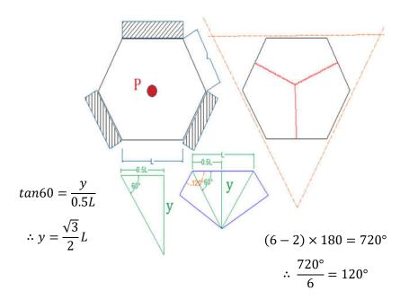
**EXAMPLE 27:** Using the yield line theory, determine the ultimate resisting moment per linear meter (m) for the isotropic reinforced two-way slab sustaining a uniformly distributed load of 9kN/m<sup>2</sup> and a line load of 5kN/m as shown in the figure below.
