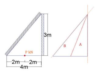
**EXAMPLE 22:** For the fixed two-way slab shown below, using the yield line theory determine the ultimate resisting moment per linear meter (m) if the slab was subjected to a concentrated load of P kN.
