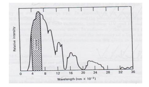
Figure 1. Relative intensity of solar energy of different wavelength at the earth's surface.
