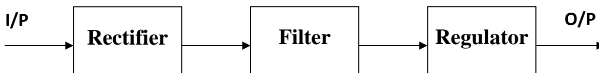
Fig (12-1) Block diagram showing part of power supply
