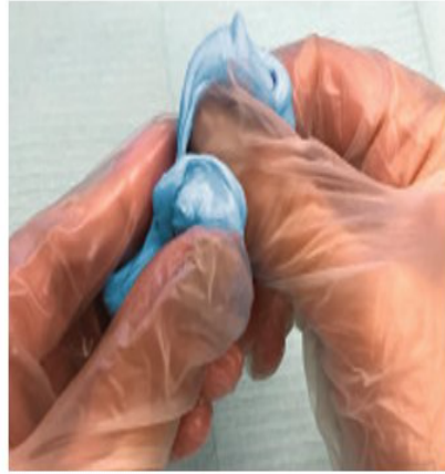
Knead the FLEXCEED base & catalyst until a uniform blue color is achieved
