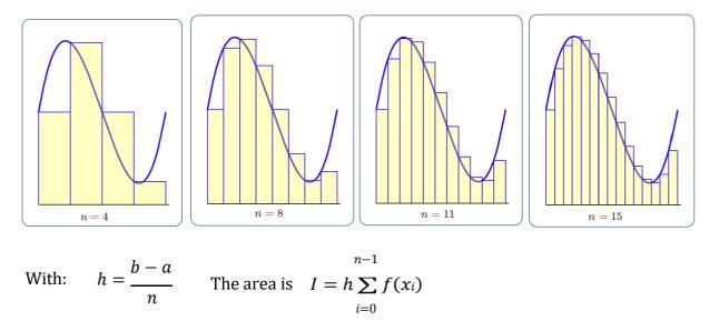
**Example1:** Calculate the following integral using rectangular rule. Use n = 6.
