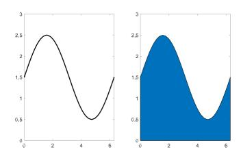
The integration of this equation over the indicated period is the area under the curve:
