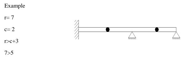
The beam is indeterminate 2<sup>nd</sup> degree if stable
