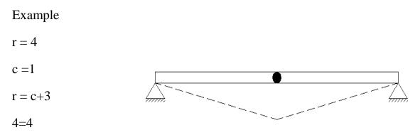
The beam is unstable because the Internal geometric instability
