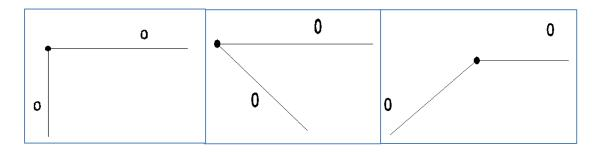
2- When met three bars in joint two of them on one straightness and there is no external force on this joint, we conclude that the force in third bar equal to zero.
