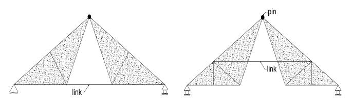
iii- A pin and two links intersecting at support
