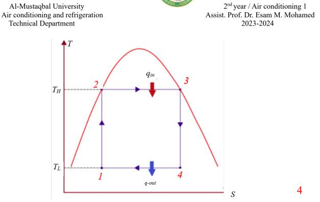
if we were to reverse the cycle such that instead of expansion we have compression, instead of compression we have expansion and transfer is also reversed. We obtain the carnot refregerator.
