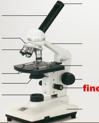
small, round knob on the side of the microscope used to fine-tune the focus of your specimen
