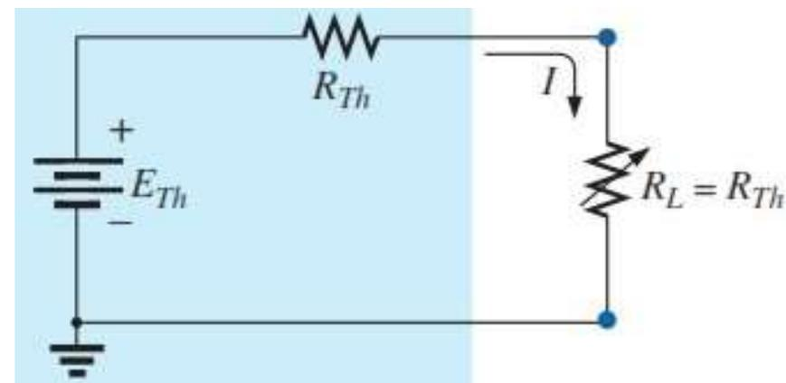
The maximum power delivered to the load can be determined by first finding the current:
