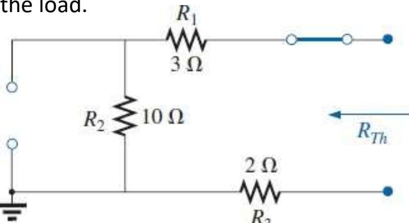
$$R_{Th} = R_1 + R_2 + R_3 = 3 \Omega + 10 \Omega + 2 \Omega = 15 \Omega$$
