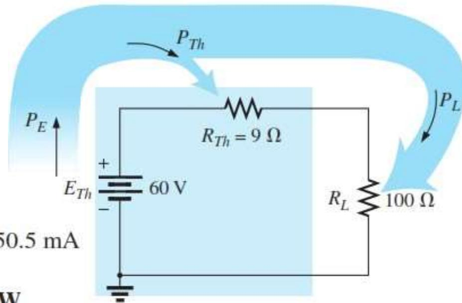
$$I_L = \frac{E_{Th}}{R_{Th} + R_L} = \frac{60\text{ V}}{9\ \Omega + 100\ \Omega} = \frac{60\text{ V}}{109\ \Omega} = 550.5\text{ mA}$$
