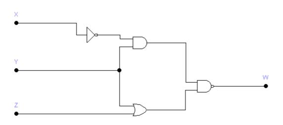
Note: the logic converter tool from EWB to fill-in the following table. For that, you need to connect the A, B and C inputs of the logic converter to X, Y and Z lines, respectively. Further, you need to connect the 'out' line of the logic converter to W. As shown in the following diagram
