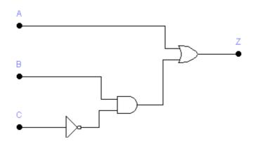
Now after drawing the circuit above using EWB we find that its truth table is as shown below (notice thatlogic **1 means connect** the input to the Vcc line, and logic **0 means connecting** the input to the ground)
