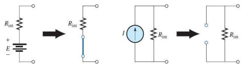
Removing a voltage source and a current source to permit the application of the superposition theorem.
