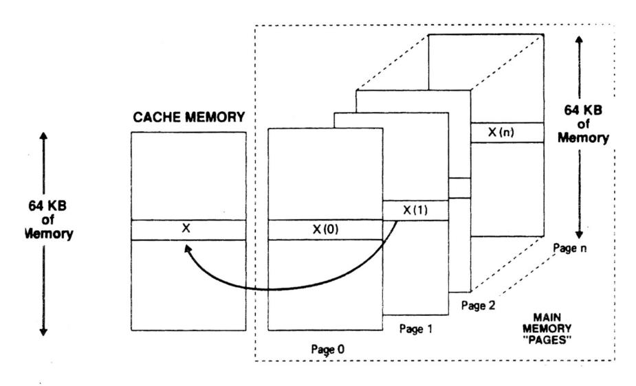
Figure 10.42 Organization of a direct-mapped memory subsystem. (Reprinted by permission of Intel Corp. Copyright/Intel Corp. 1990)
