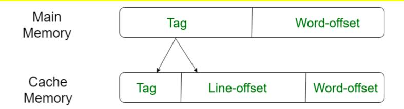
A direct cache mapping process used with 64 lines to access a memory with 4096 lines (pages) and each page / line contain 128 locations
