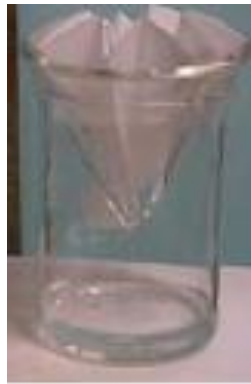
Fig.2. A beaker containing a stem less funnel. Note that the filter paper is fluted; however, that is not necessary for all applications.
