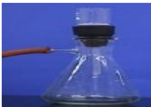
Fig. 4. A filter crucible in a crucible holder in a filter flask, with rubber tubing connected to an aspirator.
