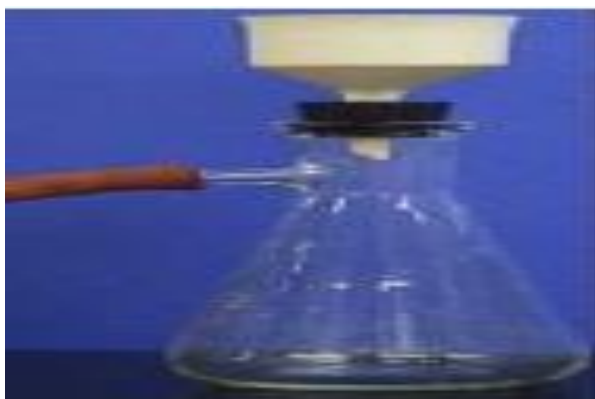
Fig. 3. A Buchner funnel in a filter flask, with rubber tubing connected to an aspirator.
