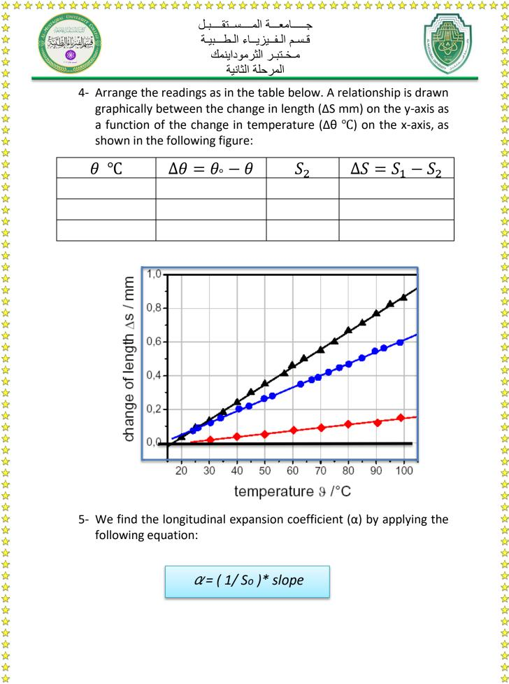
4- Arrange the readings as in the table below. A relationship is drawn graphically between the change in length ( $\Delta$ S mm) on the y-axis as a function of the change in temperature ( $\Delta \theta$  °C) on the x-axis, as shown in the following figure:
