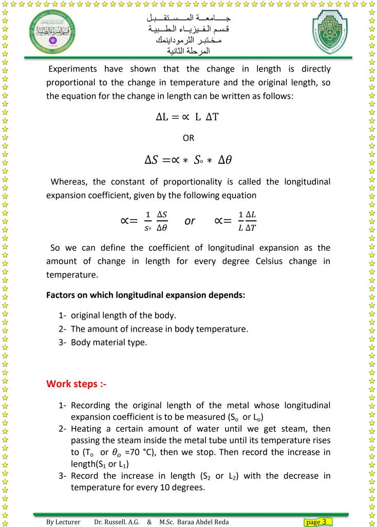
Experiments have shown that the change in length is directly proportional to the change in temperature and the original length, so the equation for the change in length can be written as follows:
