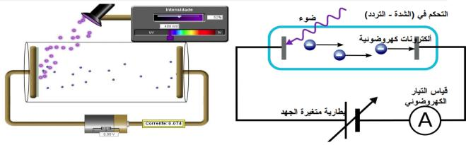
Figure 1 (The working principle of the photoelectric cell)
