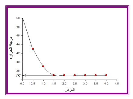
7- Calculating the heat capacity of the calorimeter taking into consideration that the specific heat of water is (1Call/g.C°) as will be shown through the calculation method attached to the experiment.
