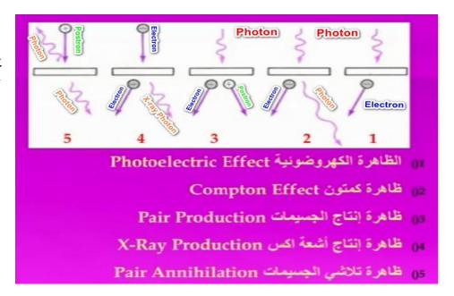
These processes lead to the absorption of a number of photons of the incident radiation, and this absorption reduces the number of photons that will transmitted from the surface.
