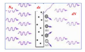
In the above figure, if  $N_0$  is the density of the incident photons on a material whose thickness is dx and the density of the photons transmitted from the material is dN, so the relationship between the change in the density of the incident photons on the material and the thickness of the material is as follows:
