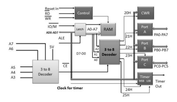
Ex: design (draw) and determine the address of the control/status, I/O ports and timer register of the 8155 if the output of decoder O2?
