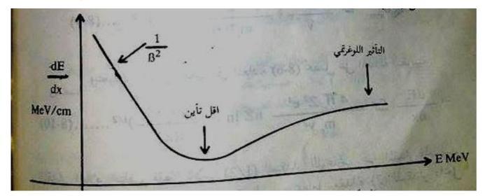
We notice from the above figure that the **stopping energy decreases as the energy of the falling particle increases** (i.e., its velocity), so that the amount of
