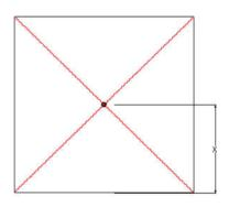
**EXAMPLE 6:** Using the yield line theory, determine the ultimate resisting moment per linear meter (m) for the isotropic two-way square slab supported by four concrete walls subjected to a uniformly distributed load (w).
