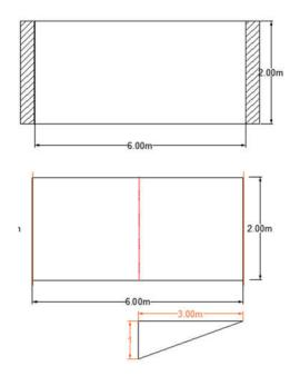
**EXAMPLE TWO:** by using the yield line theory, determine the moment for a reinforced concrete one-way slab with a length of 6m and width of 2m and is supported by two concrete walls at its width subjected to a distributed load of (w).
