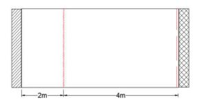
**EXAMPLE 4:** Using the yield line theory, determine the ultimate resisting moment per linear meter (m) for the isotropic simply supported reinforced concrete two-way square slab subjected to a uniformly distributed load (w).
