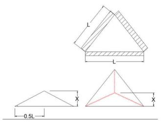
**EXAMPLE 12:** using the yield line theory, determine the moment (m) for the isotropic reinforced concrete slab subjected to a concentrated load (P).
