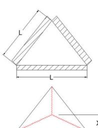
**EXAMPLE 11:** using the yield line theory, determine the ultimate resisting moment per linear meter (m) for an isotropic reinforced concrete slab simply supported at all edges and subjected to uniformly distributed load (w).
