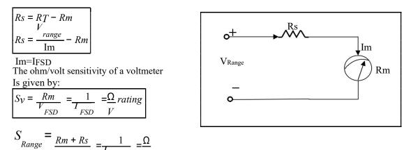
So the internal resistance of voltmeter or the input resistance of voltmeter is
