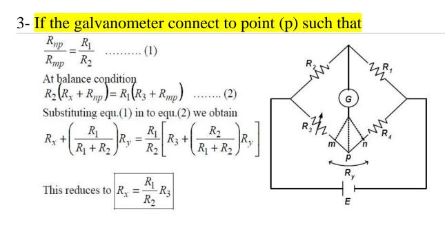
So the effect of the resistance of the connecting lead from point (m) to point (n) has be eliminated by connecting the galvanometer to the intermediate position (p).
