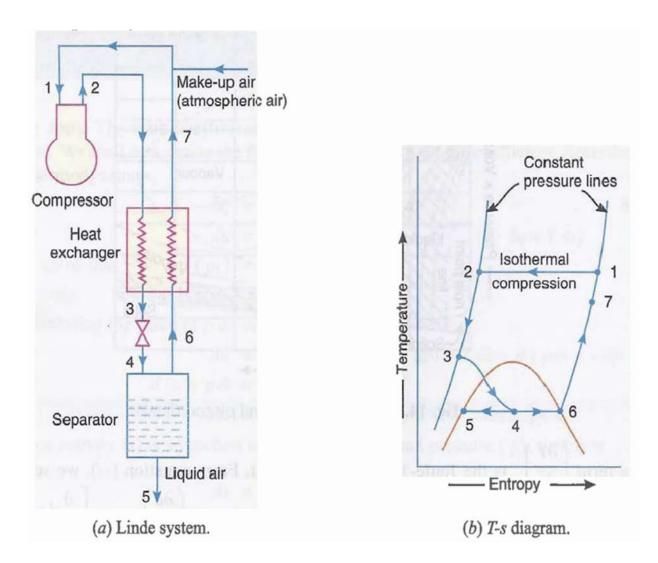
Now for the heat balance of the heat exchanger,
