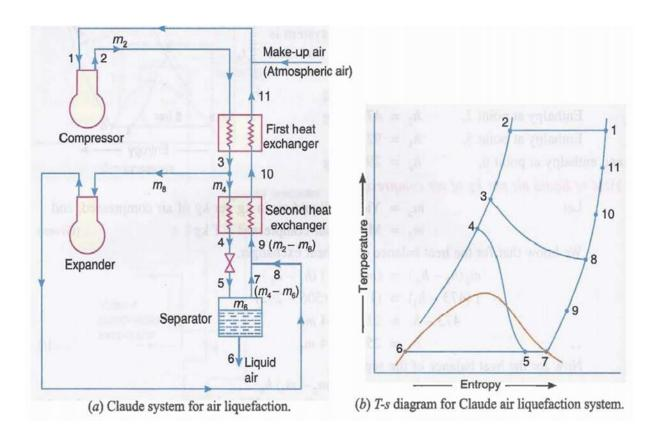
Now for the heat balance of the first heat exchanger,  $m_2(h_2-h_3) = (m_2-m_6) \ (h_1-h_{10})$  For the heat balance of the second heat exchanger  $m_4(h_3-h_4) = (m_2-m_6) \ (h_{10}-h_9)$  and for the heat balance of the separator,  $m_4h_5 = m_6h_6 + (m_4-m_6) \ h_7$
