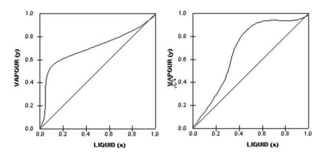
The most intriguing VLE curves are generated by azeotropic systems. An azeotrope is a liquid mixture which when vaporized, produces the same composition as the liquid. The two VLE plots below, show two different azeotropic systems, one with a minimum boiling point and one with a maximum
