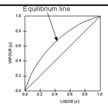
This particular VLE plot shows a binary mixture that has a uniform vapourliquid equilibrium that is relatively easy to separate. The next two VLE plots below on the other hand, shows non-ideal systems which will present more difficult separations.
