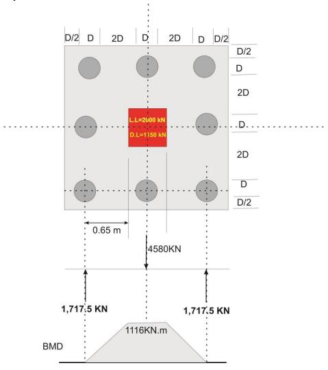
$$L = \frac{D}{2} + D + 2D + D + 2D + D + \frac{D}{2} = 8D = 8 * 300m = 2400mm$$
